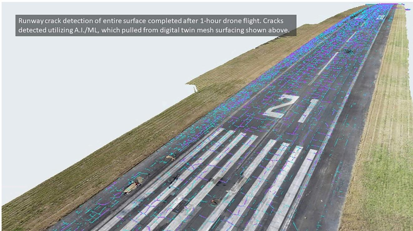
Runway crack detection of entire surface completed after 1-hour drone flight. Cracks detected utilizing A.I./ML, which pulled from digital twin mesh surfacing shown above.
